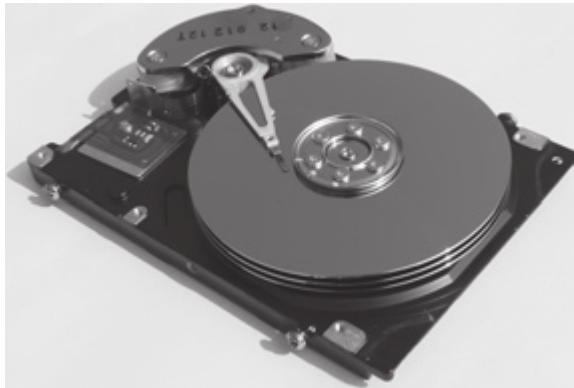
Figure 6-3: An opened hard disk drive, showing the disk heads. Photo courtesy of Geni via Wikimedia Commons, reproduced under CC BY-SA 4.0 ( https://creativecommons.org/licenses/by-sa/4.0/ ).
