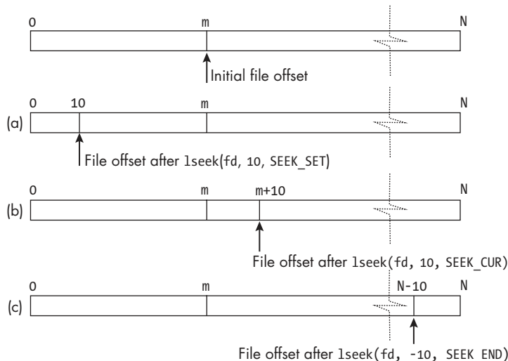
Figure 5-2: The effect of the whence parameter on the movement of the file offset. In (a) it's moved using whence = SEEK_SET , in (b) using whence = SEEK_CUR , and in (c) using whence = SEEK_END .
