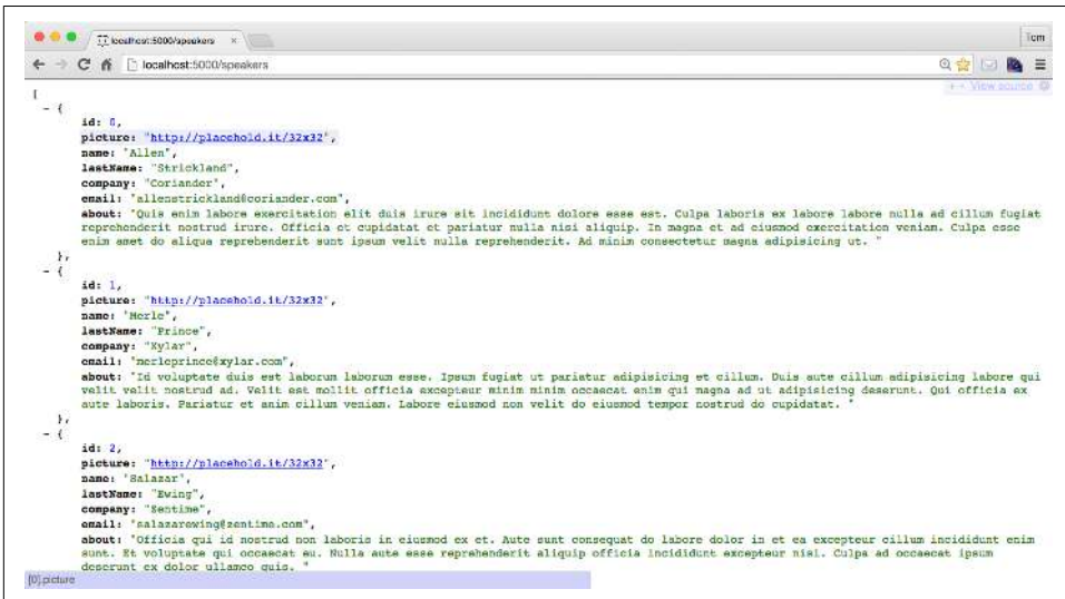
Figure 5-11. Speakers Stub API on json-server
