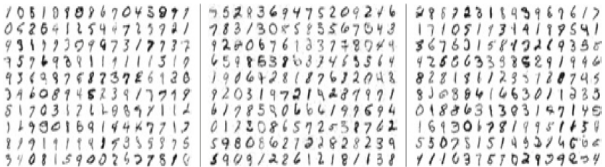
Figure 17-5: The generated DCGAN digits for latent vector dimensions 10, 80, and 160 (left to right)
