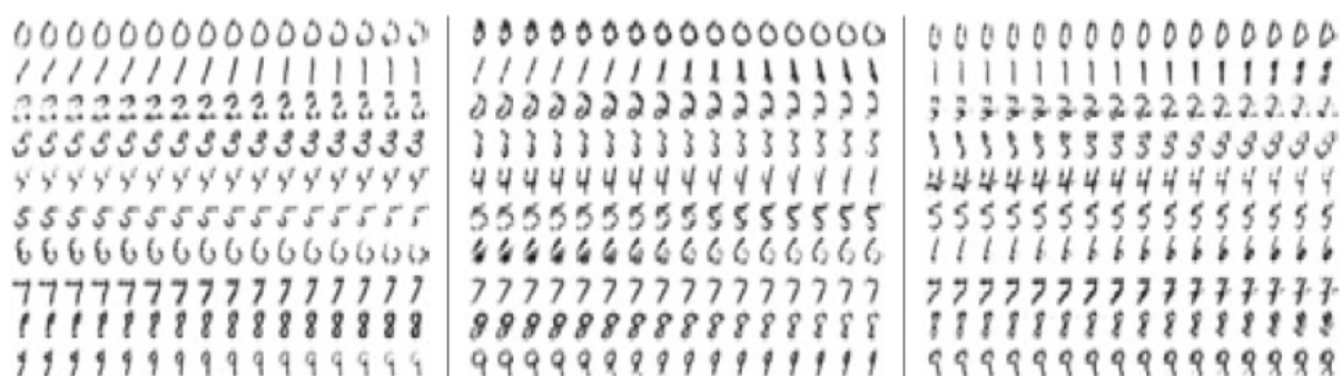
Figure 17-10: Interpolations along random directions in the 10-dimensional latent space
