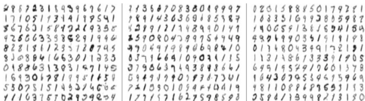
Figure 17-6: The generated DCGAN digits for 160-dimensional latent vectors for 12,000, 24,000, and 36,000 iterations (left to right)
