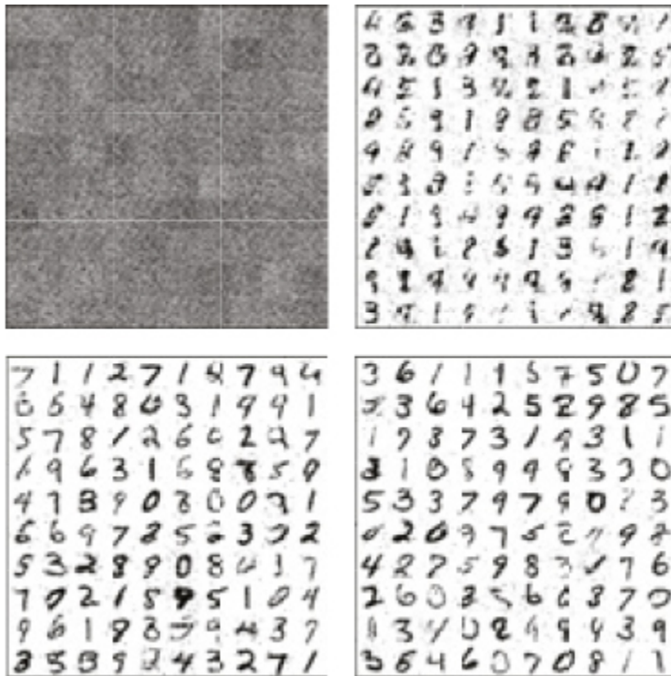
Figure 17-4: The results of training an MLP-only GAN: iterations 1 and 2,000 (top); iterations 30,000 and 80,000 (bottom)
