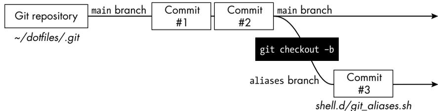
Figure 18-5: The `git checkout -b` command creates a new `aliases` branch to which you commit the `git_aliases.sh` file.
