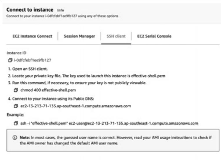
Figure 22-9: Instructions for connecting to the virtual machine
